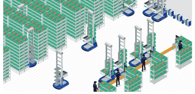
Fig. 1. The MTSR autonomous mobile robot system, where robots directly pick multiple totes from vertical storage shelves [7].
