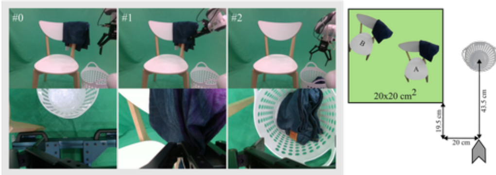
(e) Place Jeans to Basket: The robot base ( F_R ) is fixed relative to the laundry basket. The jeans is semi-folded and hanging on the right edge of the chair. The chair position is randomized in the 20\text{ cm} \times 20\text{ cm} region. The robot grasps the jeans from the side and places it in the laundry basket. We collected 50 demonstrations, in each half of the demonstrations the chair position is randomized keeping the orientation A and in the other half the orientation of the chair remained B. The average length of the demo is 592 steps or 44 secs.
