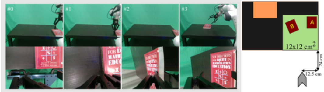
(h) Slide Book and Pick Up: The robot base ( F_R ) is fixed relative to the black coffee table. The book position is randomised in the 12\text{ cm} \times 12\text{ cm} region. In half of the demonstrations, the book orientation is kept A and in the other half, orientation B. The robot first corrects the book orientation if necessary by pushing on its edge and then slides the book to the edge of the table. It then picks it up and places it in the area depicted by orange (rightmost figure). We collect 50 demonstrations in total with an average demo length of 930 steps or 70 secs.
