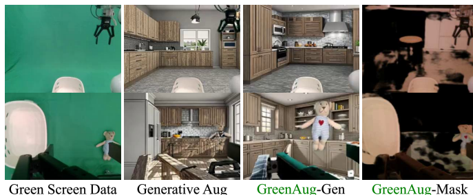
Figure 5: Visualisations of raw and preprocessed frames (left shoulder and lower wrist camera views) of generative augmentation, GreenAug-Gen and GreenAug-Mask (during inference). Both generative methods struggle with producing good contextual wrist camera inpainting. In generative augmentation, the gripper is inpainted as part of the background, while GreenAug-Mask shows masking artefacts in novel scenes.
