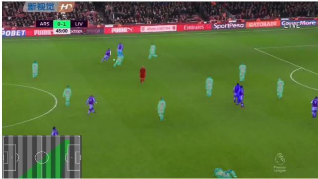
Figure 3: Illustration of the segmentation, team cluster and view transform results. The translucent mask represents each player’s segmentation results and the color of mask represents different teams, including judges’ color. The court map on the left bottom corner represents camera view field after transformed from the original image.
