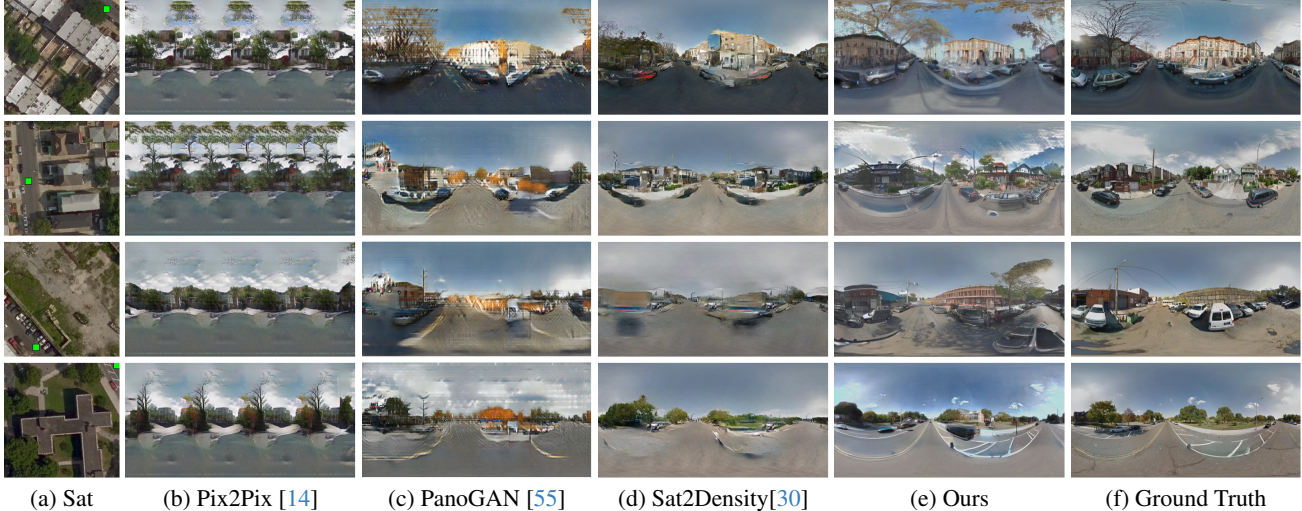
Figure 6. Qualitative results versus baselines. The cross-view synthesis methods that we compare with are trained on our collected center-aligned satellite images. Our approach, which integrates nearby street-level panoramas, not only generates more realistic results when compared to baselines, but more accurate results both semantically and geometrically when compared to the ground truth.
