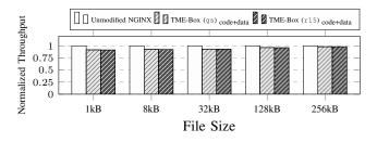
Fig. 9: Throughput of NGINX with TME-Box for requesting different file sizes normalized to the unmodified NGINX.
