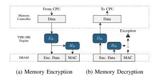
Fig. 2: Overview of TME-MK's memory encryption with integrity support. Memory operations leverage a specific encryption key that is determined by the keyID to encrypt and decrypt data located in DRAM. Memory accesses using an incorrect keyID are detected by a MAC mismatch and result in a hardware exception.
