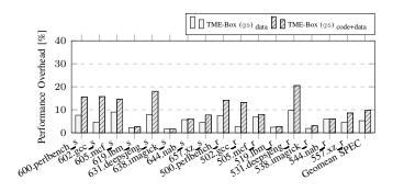
Fig. 7: The relative performance overhead of TME-Box using the qs-mode for the SPEC CPU2017 benchmark suite.
