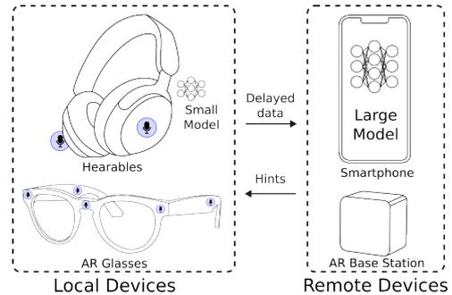
Figure 1: Example use cases for knowledge boosting. During inference, small models running locally can benefit from the knowledge capacity of large models running remotely. In these examples, the communication latency between the local and remote devices can exceed the real-time processing requirements.
