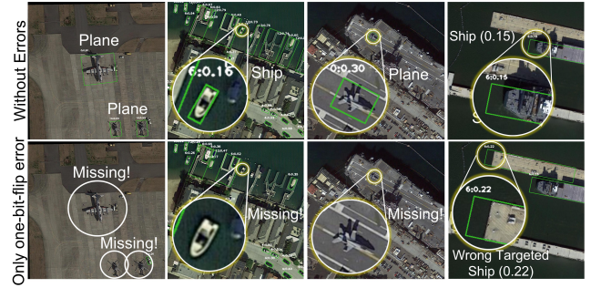
Figure 8: 1-bit error in Task 5 (YOLO) leads to wrong results.
