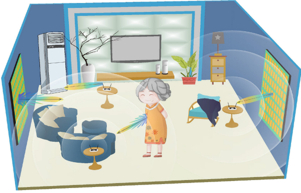
Fig. 1. A scenario for smart and cost-effective wireless imaging of the elderly indoors involves installing dual-RIS integrated into the walls of living rooms or hallways. This system serves as a complementary method to cameras in scenarios with low light, line-of-sight obstructions, and privacy concerns.
