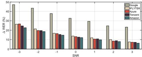
Figure 8. Robustness of commercial ASRs against white noise
