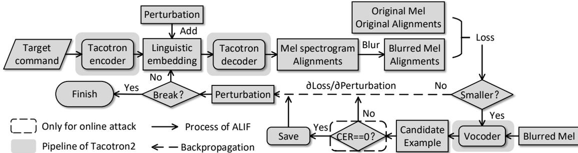
Figure 6. Architecture of the ALIF-OTL scheme. The scheme is based on the ALIF pipeline shown with a solid line.
