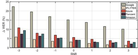
Figure 9. Robustness of commercial ASRs against event noise
