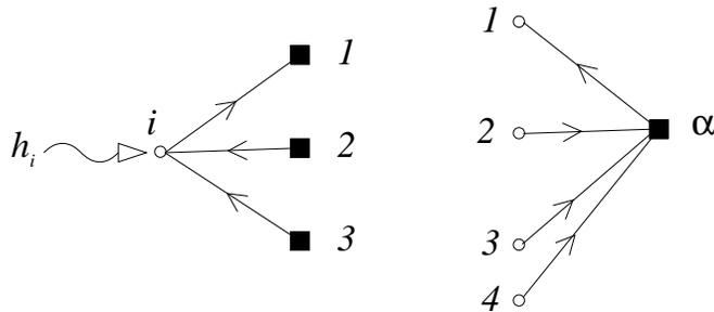
Figure 4: A graphic representation of the operations executed in a message passing algorithm. At the variable node  $i$  (on the left):  $x_{i \rightarrow 1}^{(t+1)} = F(y_{2 \rightarrow i}^{(t)}, y_{3 \rightarrow i}^{(t)}; h_i)$ . At the check node  $\alpha$  (on the right):  $y_{\alpha \rightarrow 1}^{(t+1)} = G(x_{2 \rightarrow \alpha}^{(t)}, x_{3 \rightarrow \alpha}^{(t)}, x_{4 \rightarrow \alpha}^{(t)})$ .
