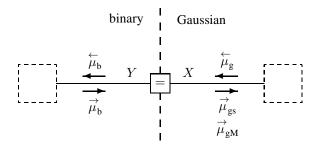
Fig. 2. Converting a soft-bit message  $\vec{\mu}_{b}$  into a Gaussian message  $\vec{\mu}_{gs}$  or  $\vec{\mu}_{gM}$ .
