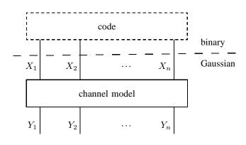
Fig. 3. Joint code/channel factor graph.
