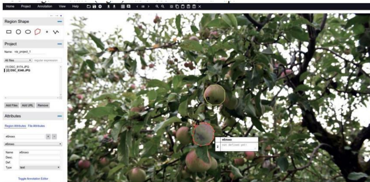
Figure 2: The process of marking up data and highlighting image classes in VGG Image Annotator
