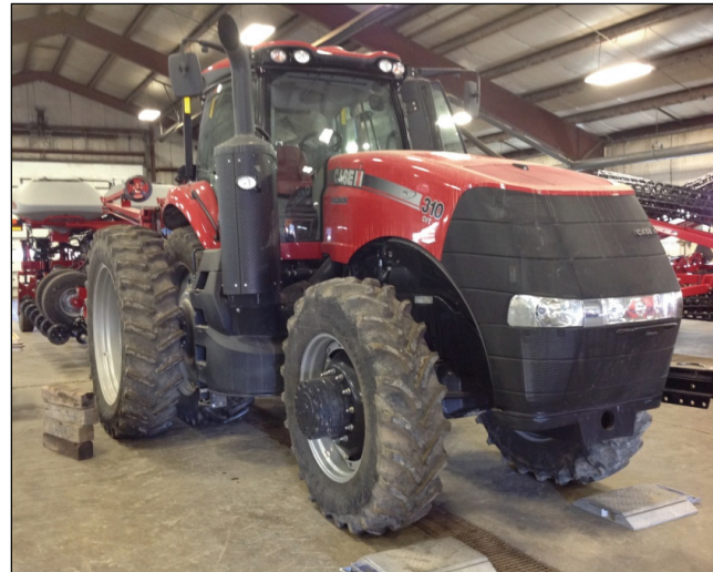
Figure 3. Case IH Magnum 310 tractor with 16 row Case IH 1255 planter being weighed in spring 2016.
