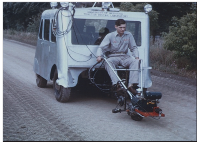
Figure 8. Test 449—the Choremaster, 0.7 drawbar HP.
