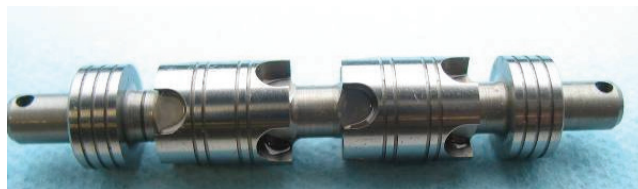
Figure 4.3. Precision machined spool used in electro-hydraulic valves.
