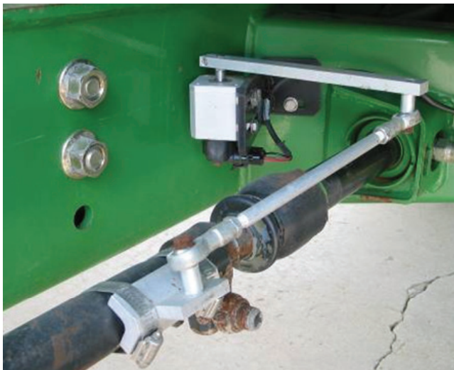
Figure 4.9. Steering angle sensor measuring cylinder extension in a combine.
