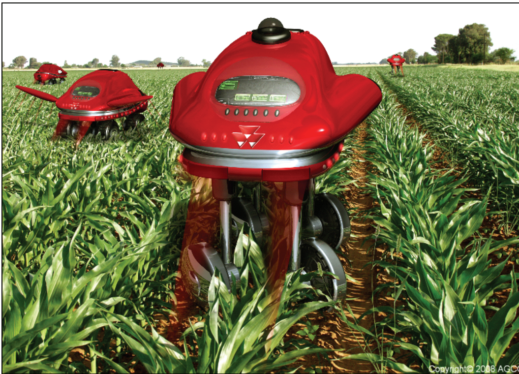
Figure 7.2. A swarm of small autonomous vehicles scouts a field (used with permission of Prof. Simon Blackmore).
