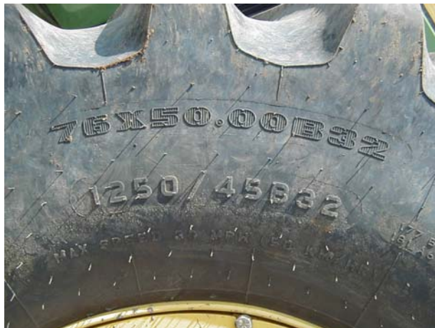
Figure 5. Flotation size designation.
