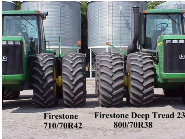
Figure 10. 710/70R42 tires versus 800/70R38 tires.
