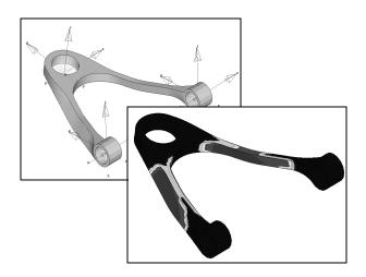
Figure 12. Finite Element Analysis.
