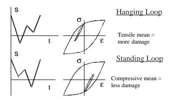
Figure 6. Illustration showing the effect of cycle sequence.
