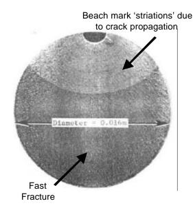
Figure 4. Beach marks (striations) on a fatigue fracture surface.
