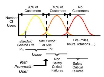
Figure 15. Durability Targets for 90th Percentile Customer.
