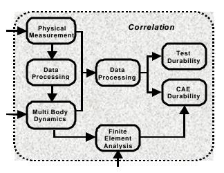
Figure 8. A Durability Process.
