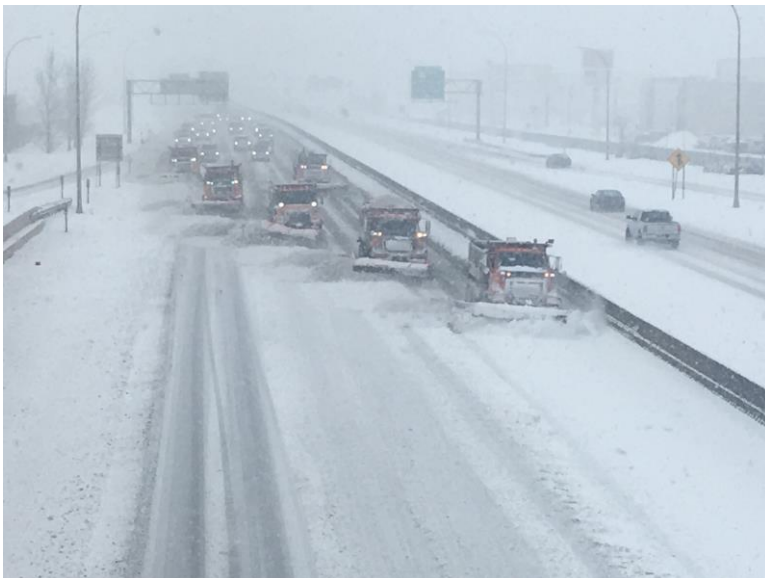
(a) Gang plowing by the Minnesota Department of Transportation (MnDOT).
