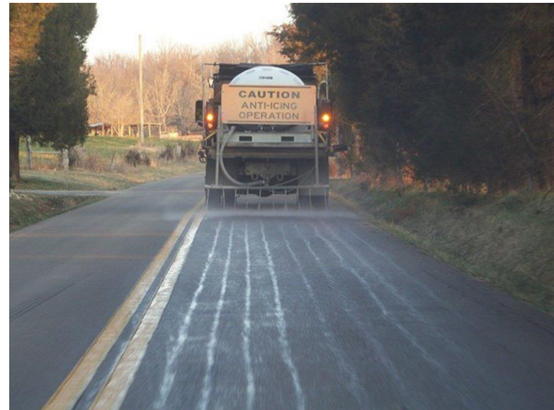
(b) Anti-icing operation by Kentucky Transportation Cabinet (KYTC).
