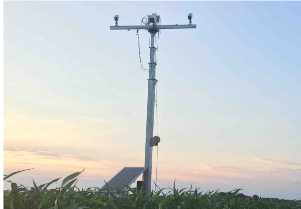
Figure 1: Observation tower with stereo RGB rig and a thermal camera centered in between
