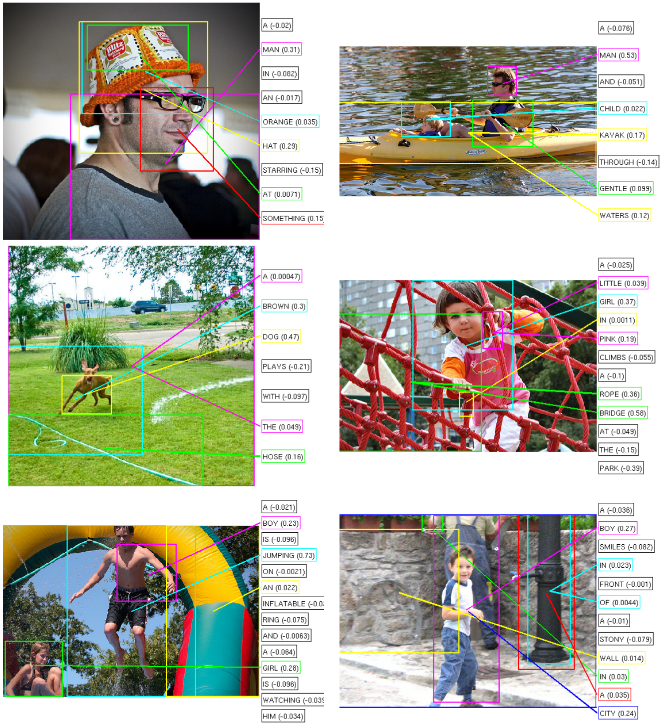
Fig. 4. Some examples of inferred alignments on the Flickr8k data. The words for each image’s caption are stacked to the right of each image, accompanied by their alignment scores. To keep the images free from too much clutter, we threshold the scores at 0, displaying a link between the word and its maximally associated object bounding box only when its score is positive. Note that the system does not actually see the text of the caption words - only a spectrogram. We replace the spectrogram in these figures with the ground truth text for the sake of clarity.
