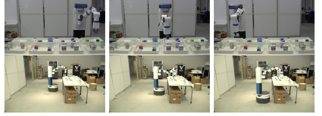
Fig. 13: (Left) Move to P_{B_1} to pick up a part from tray_1 . (Middle) Move to P_{B_2} to pick up a part from tray_2 . (Right) Move to P_{B_4} to pick up a part from tray_4 .
