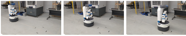
Fig. 12: Test the base positioning accuracy and repeatability by looping the mobile manipulator between two fixed positions, the black tape on the ground marks the profile of mobile base in these two positions.
