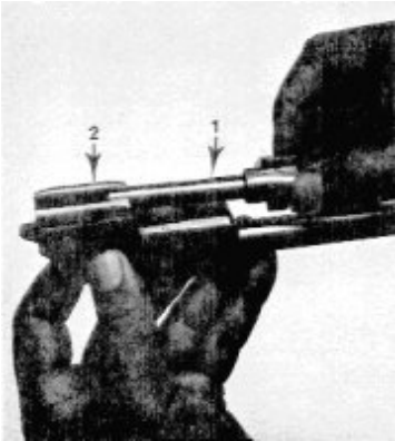
FIGURE 38. REPLACING THE BOLT 1. SPINDLE 2. CARRIER
