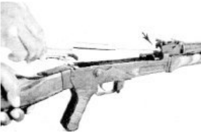
FIGURE 40. REPLACING BOLT CARRIER
